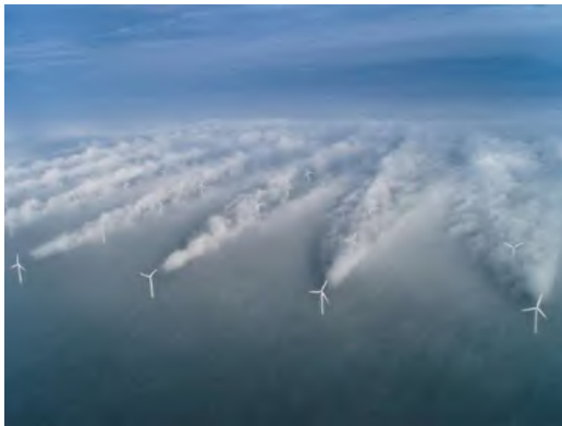
Figure 4. Photo illustration of a turbine wake effect visualised with the aid of a mixing cloud. Reproduced from NOAA ( https://www.climate.gov/news-features/featured-images/wind-turbines-churn-air-over-north-sea ). The wake formation drives the formation of liquid condensation mixing cloud.
